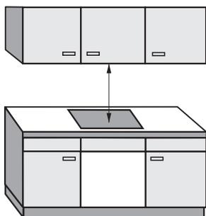
If there is more than one appliance installed below the exhaust hood, each with a different safety clearance, the largest clearance must be used.
